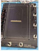
9. Place the (4) 5mm standoffs in the holes in the PCB for the screen and secure using the lock nuts.
