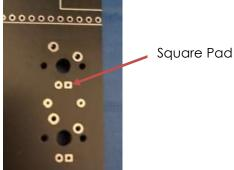
8. Solder the six Encoders on the front of the PCB as indicated (SW1-SW6)
