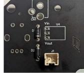
3. Solder DC Jack to bottom of PCB at CN1. Make sure jack sits square to the edge of PCB.
