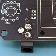
4. Solder included right angled pins to Pololu Voltage Regulator as shown below. Solder into U4 on bottom of PCB the VIN pin should be at the top of the PCB (closest to the DC jack).
